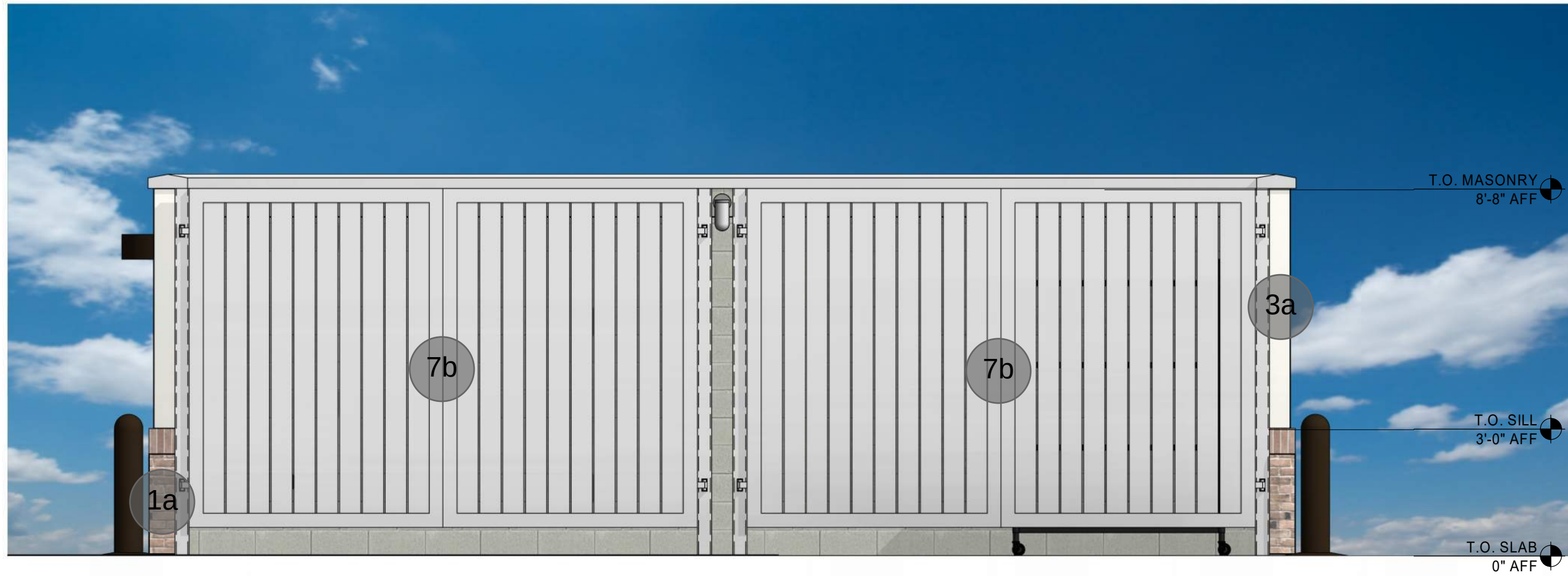
⑤ DUMPSTER FRONT ELEVATION 3/8" = 1'-0"
