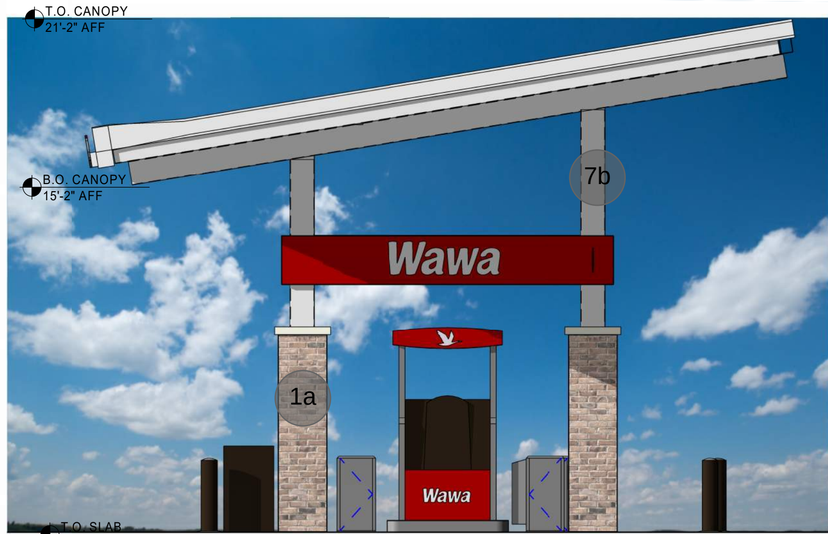
⑦ FUEL CANOPY ELEVATION 1/4" = 1'-0"
