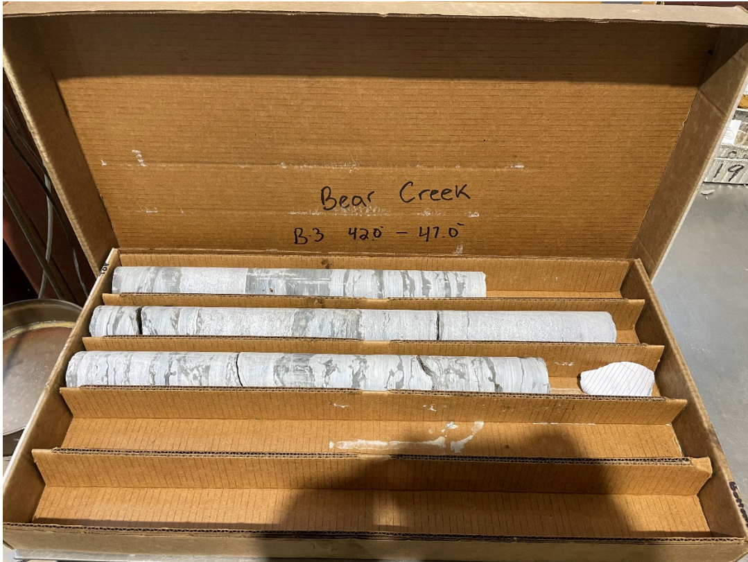
Boring B-3 rock core 42.0 feet to 47.0 feet
