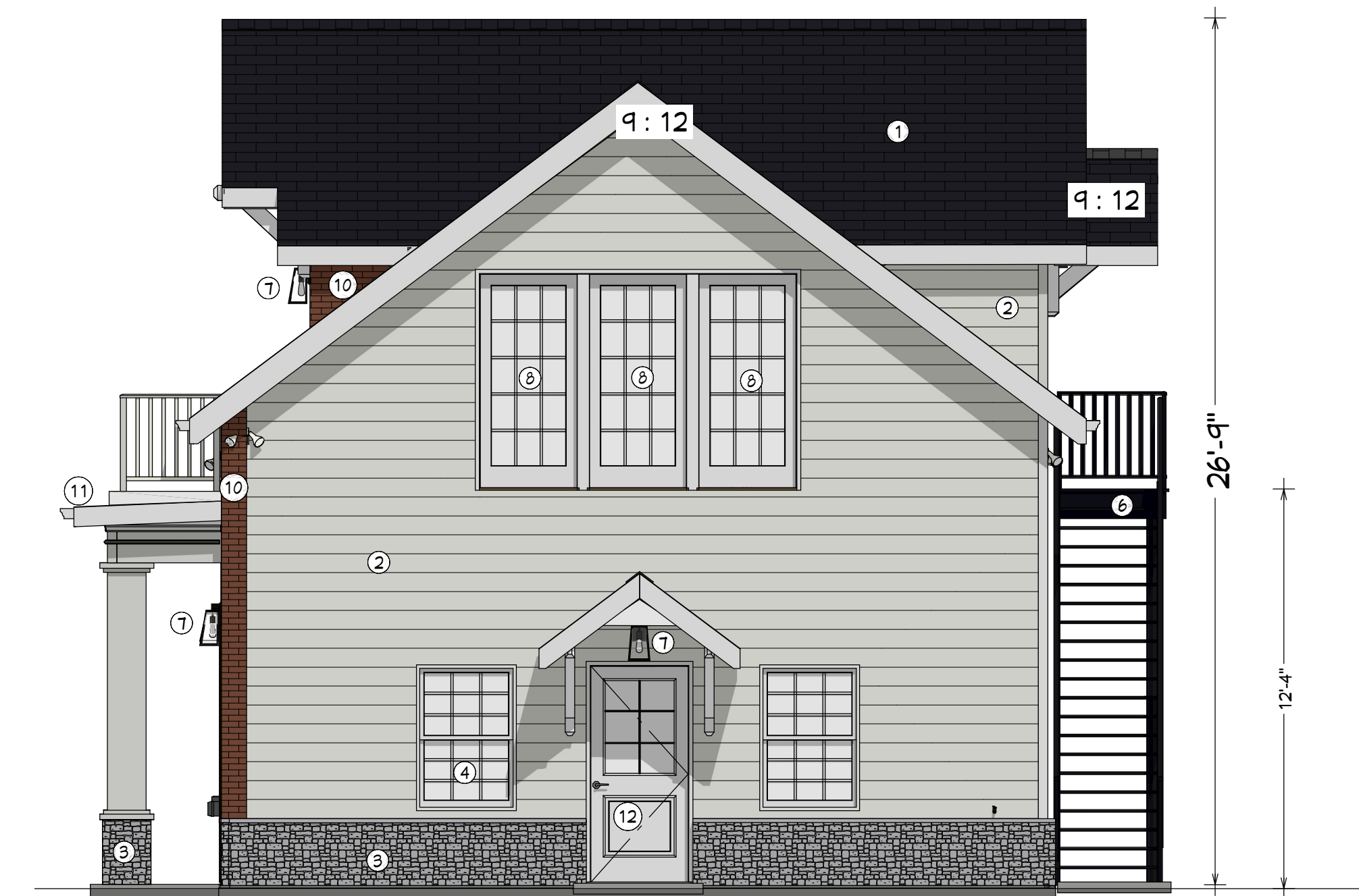
CARRIAGE HOUSE SIDE ELEVATION
