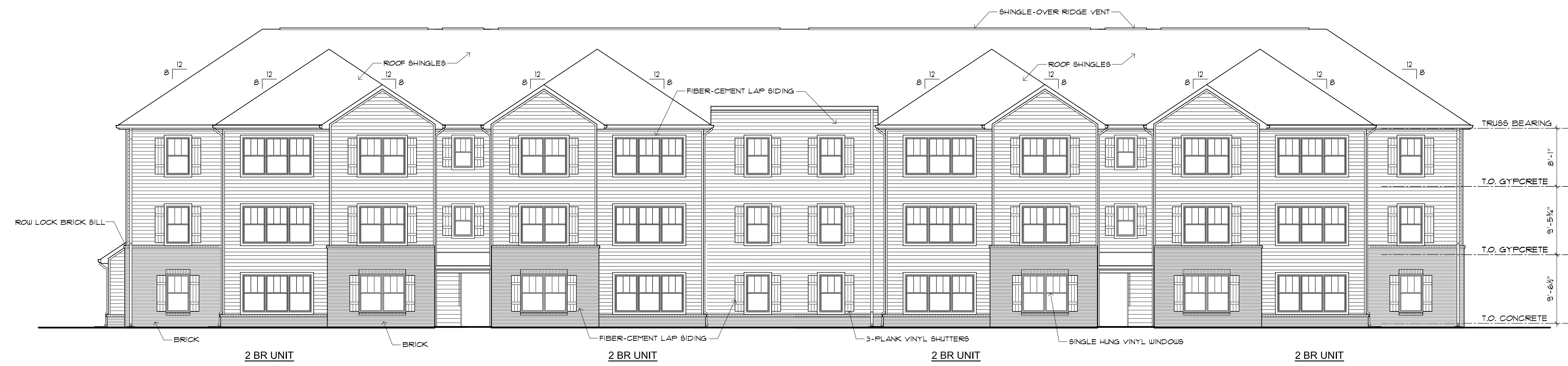
1 BUILDING C - FRONT & REAR ELEVATIONS SCALE: 1/8" = 1'-0"
