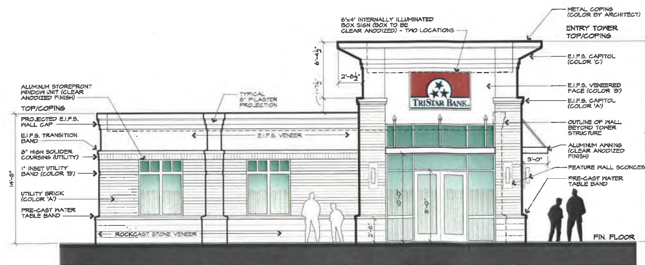
EAST BUILDING ELEVATION
