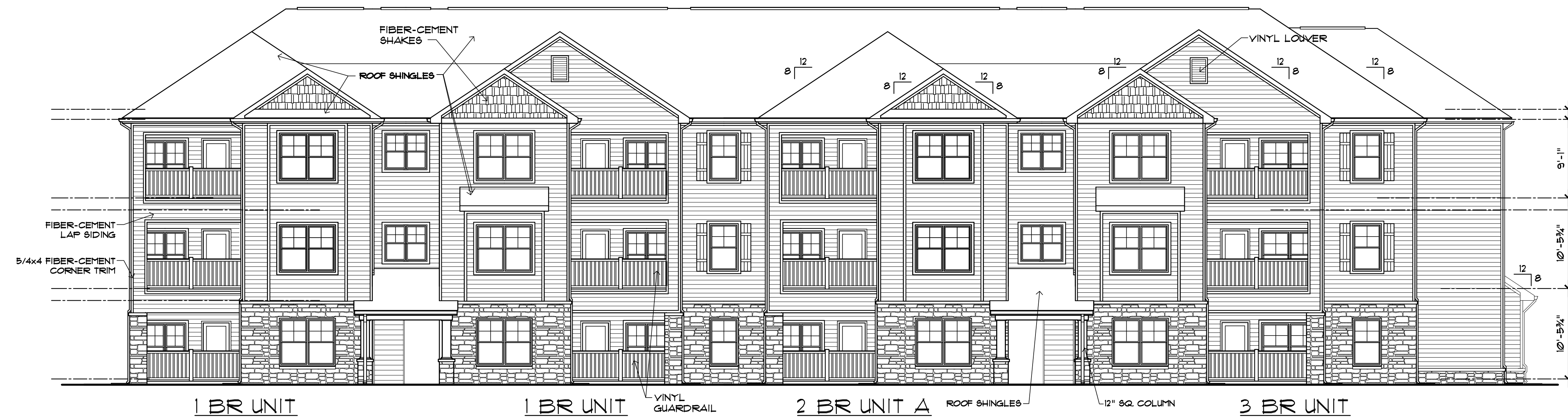
BUILDING C - FRONT ELEVATION
