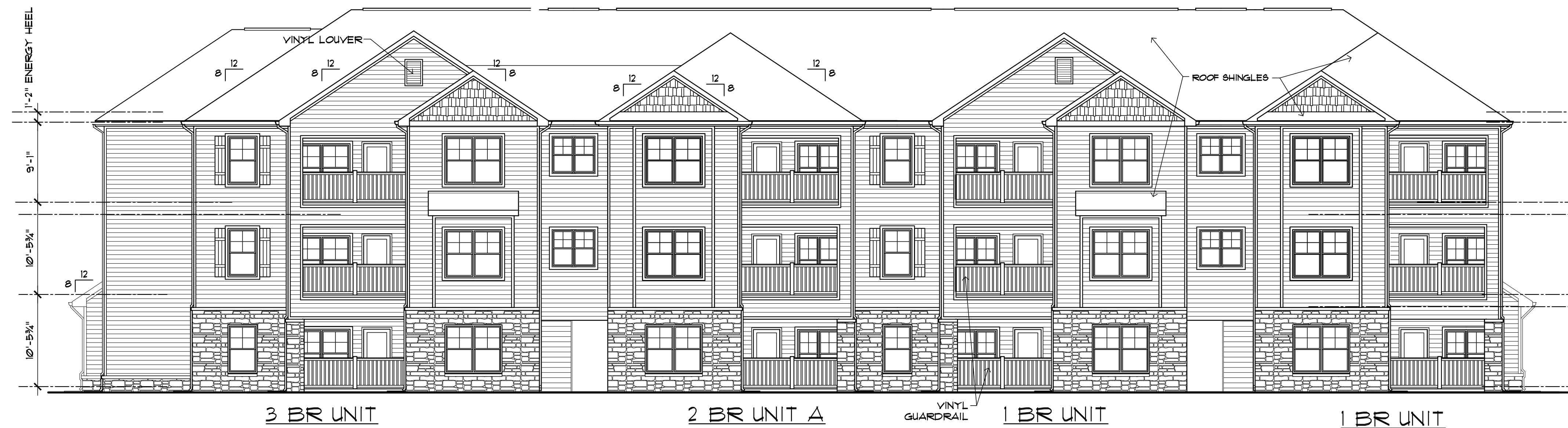
BUILDING C - REAR ELEVATION
