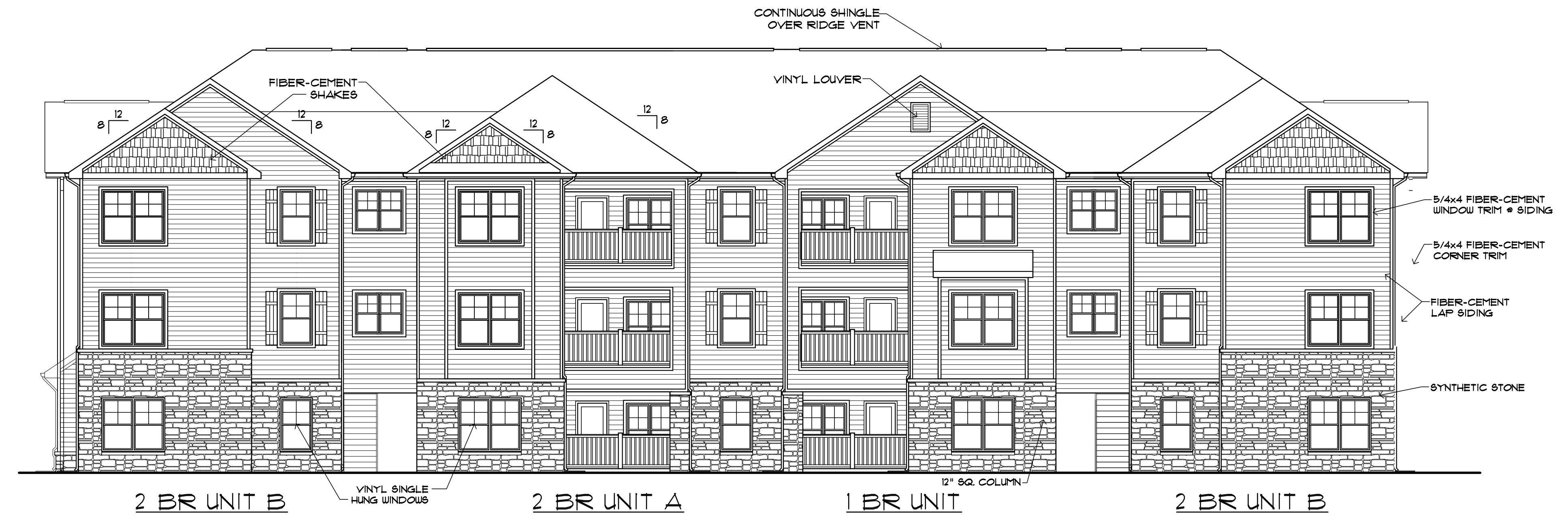
BUILDING B1 & 2 - REAR ELEVATION
