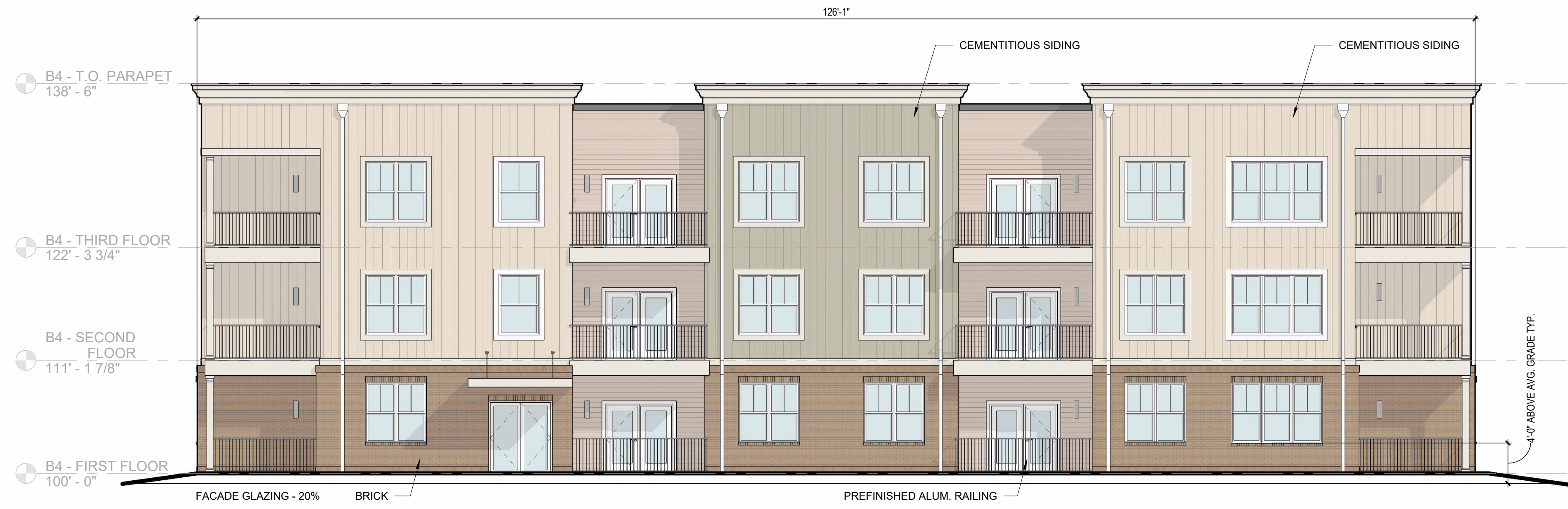
2 A204 1/8" = 1'-0" ELEVATION BUILDING 4 - (FACING WATER DETENTION AREA)
