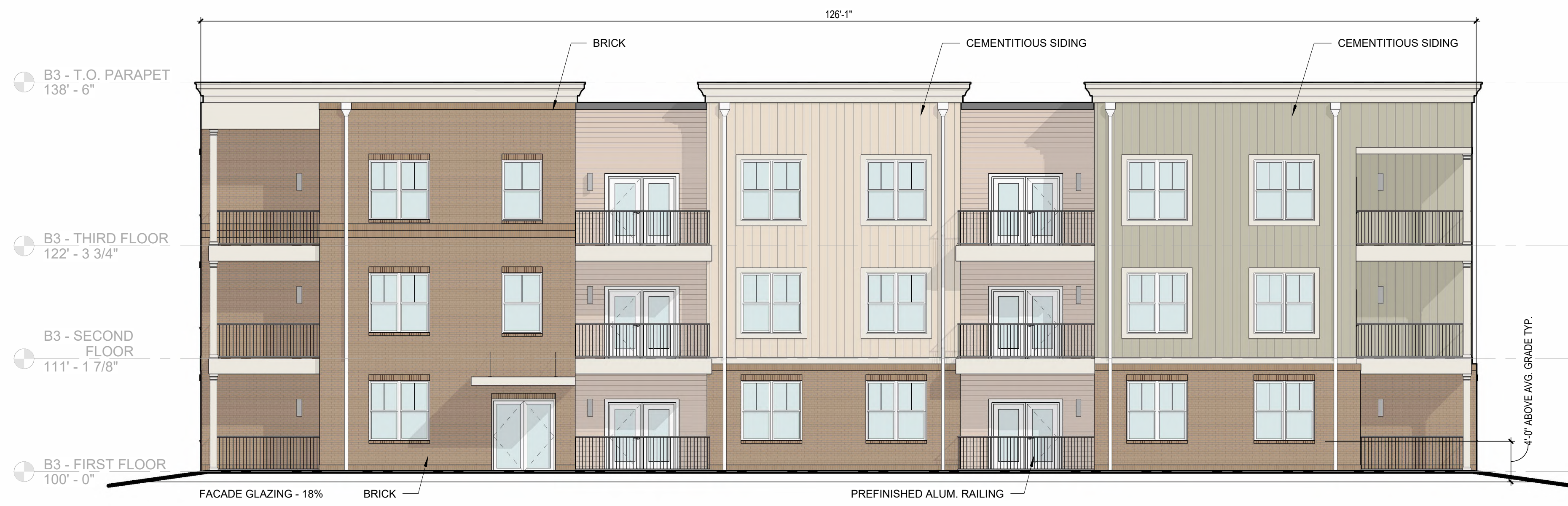
4 A203 1/8" = 1'-0" ELEVATION BUILDING 3 - (FACING BACK OF PROPERTY)
