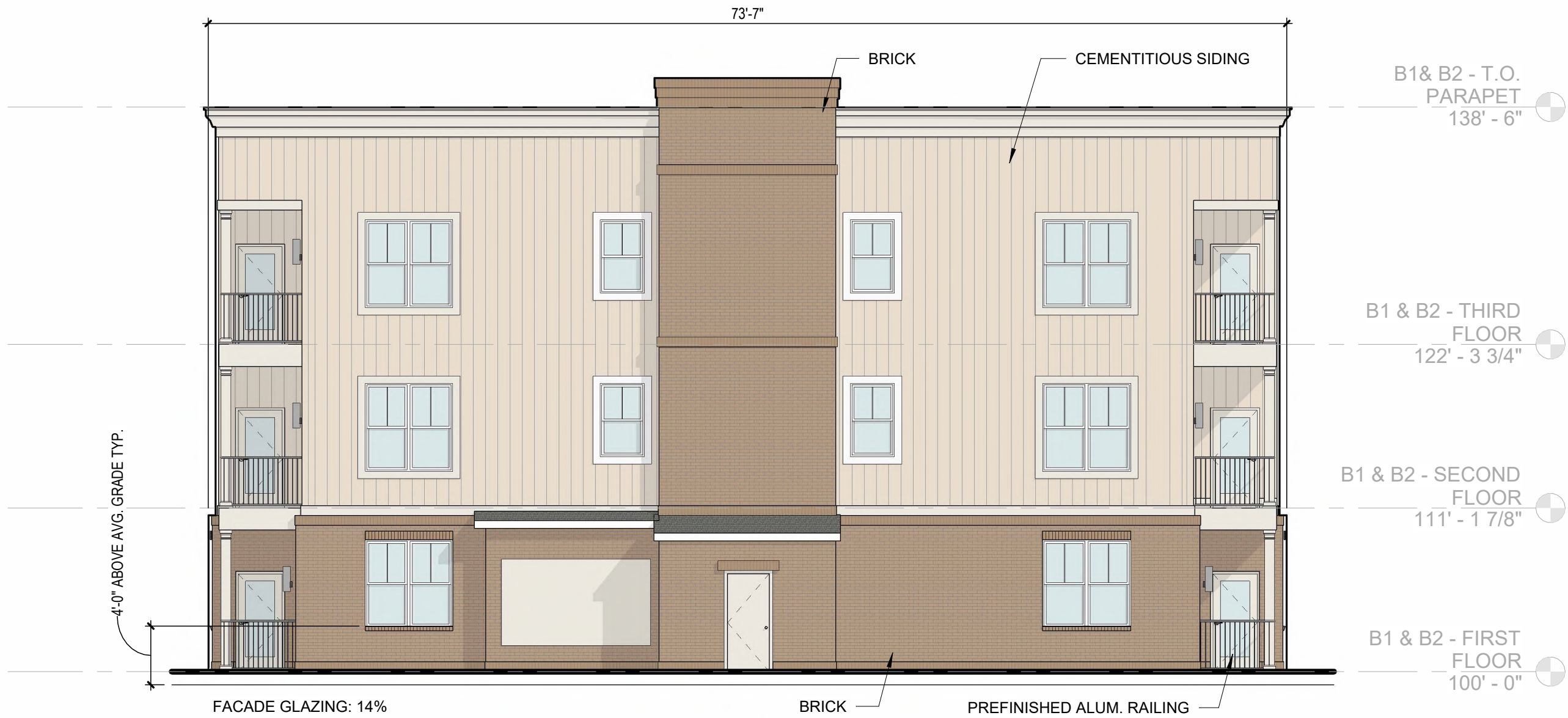
3 A201 1/8" = 1'-0" ELEVATION BUILDING 1&2 - (FACING BLDG 3)
