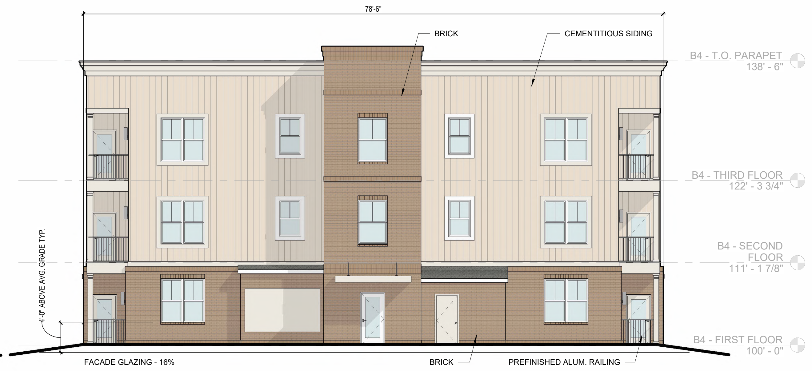
3 A204 1/8" = 1'-0" ELEVATION BUILDING 4 - (FACING BACK OF PROPERTY)
