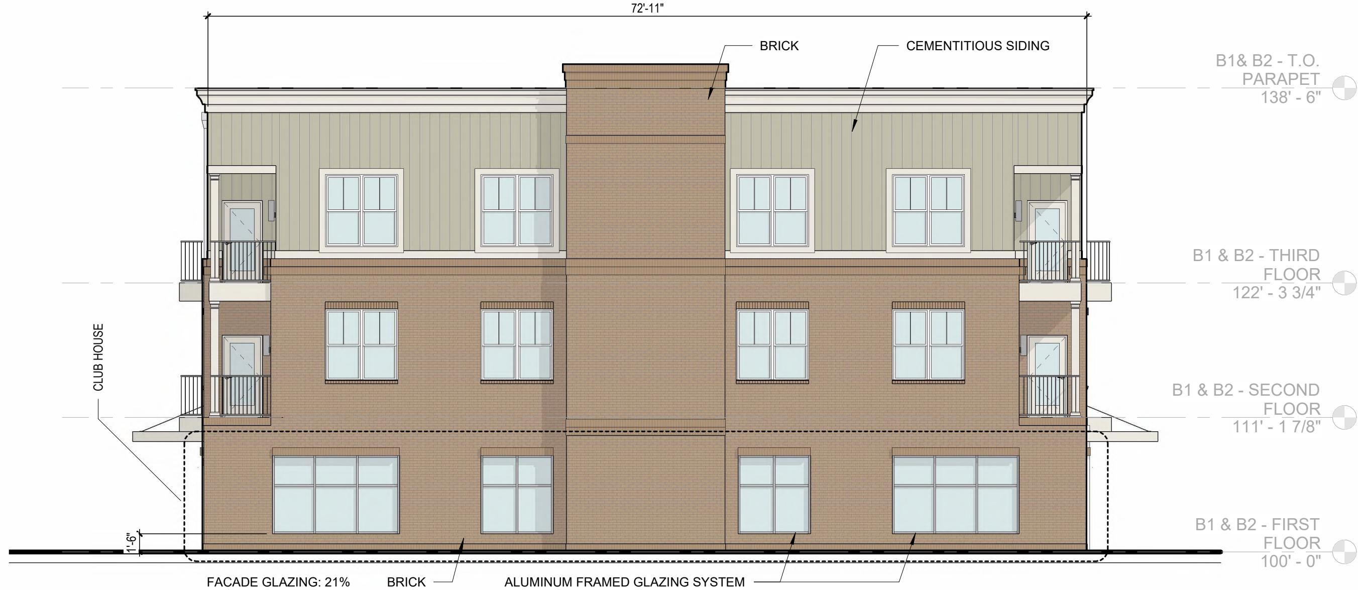
2 A201 1/8" = 1'-0" ELEVATION BUILDING 1&2 - (FACING TAYLOR'S BEND RD.)
