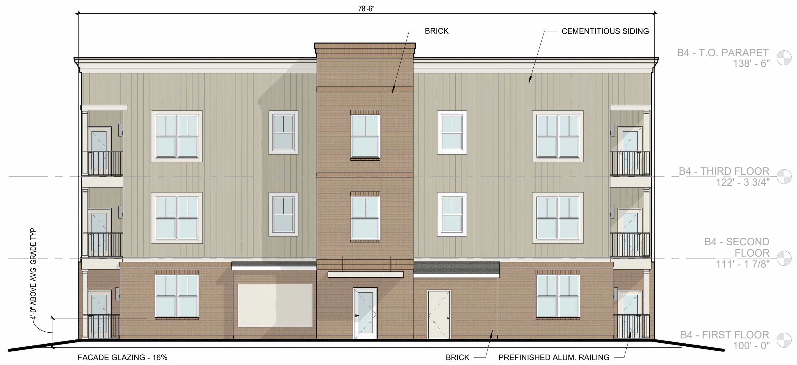
2 A203 1/8" = 1'-0" ELEVATION BUILDING 3 - (FACING PARKING LOT)
