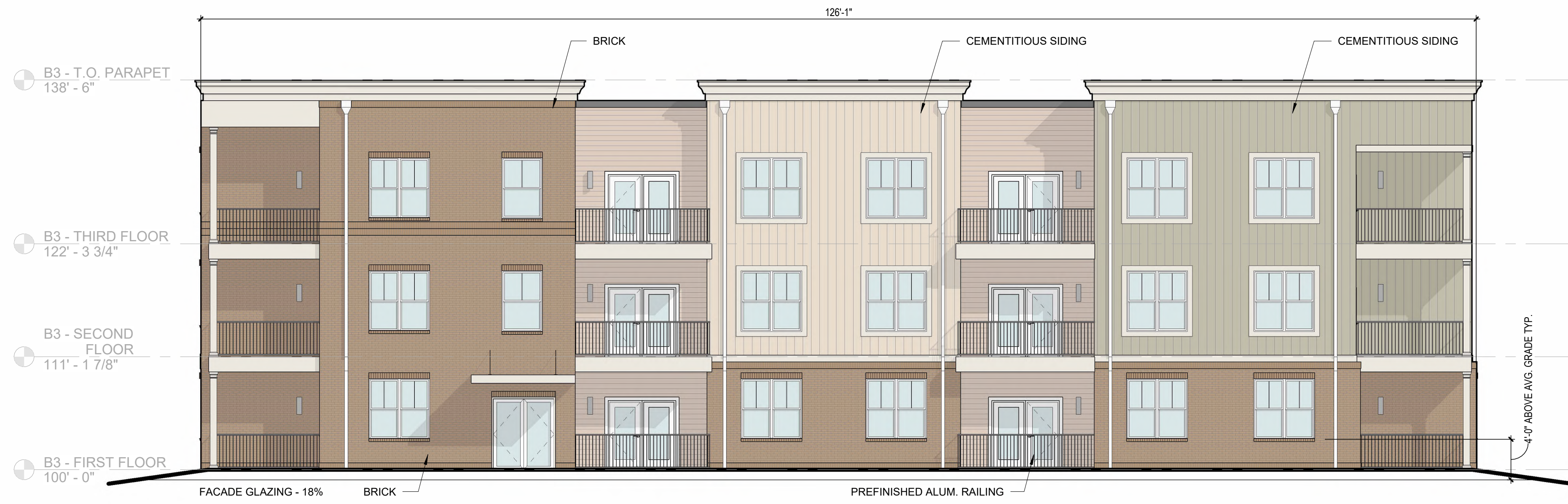
4 A203 1/8" = 1'-0" ELEVATION BUILDING 3 - (FACING BACK OF PROPERTY)
