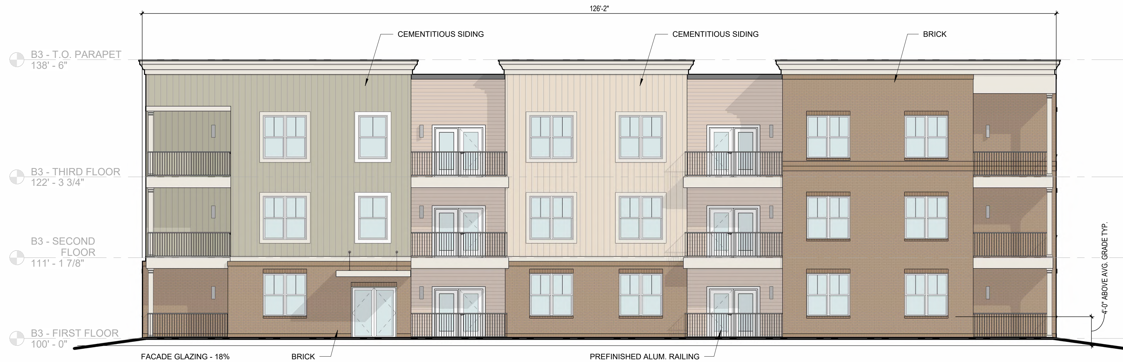
3 A203 1/8" = 1'-0" ELEVATION BUILDING 3 - (FACING BLDG 1&2)
