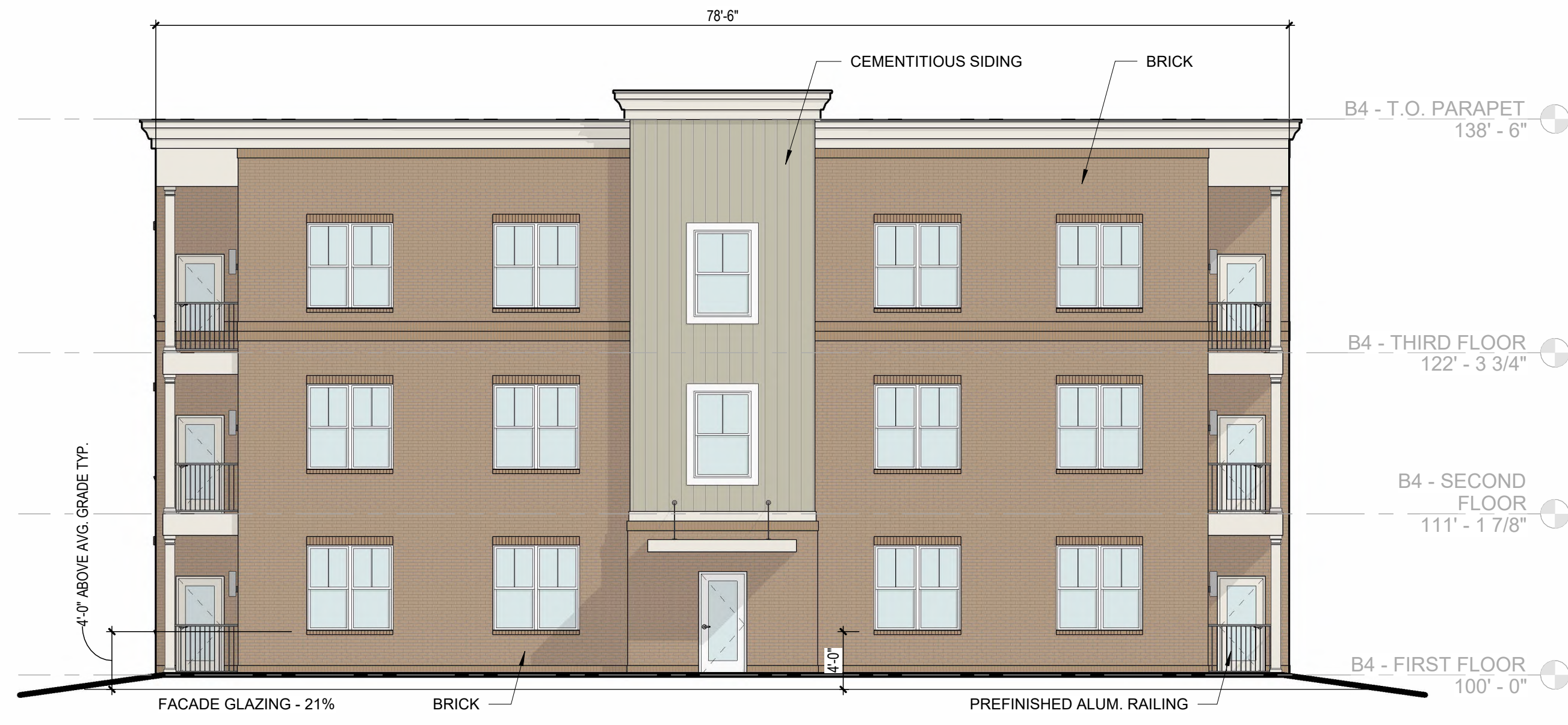
1 A203 1/8" = 1'-0" ELEVATION BUILDING 3 - (FACING RIVER RD.)
