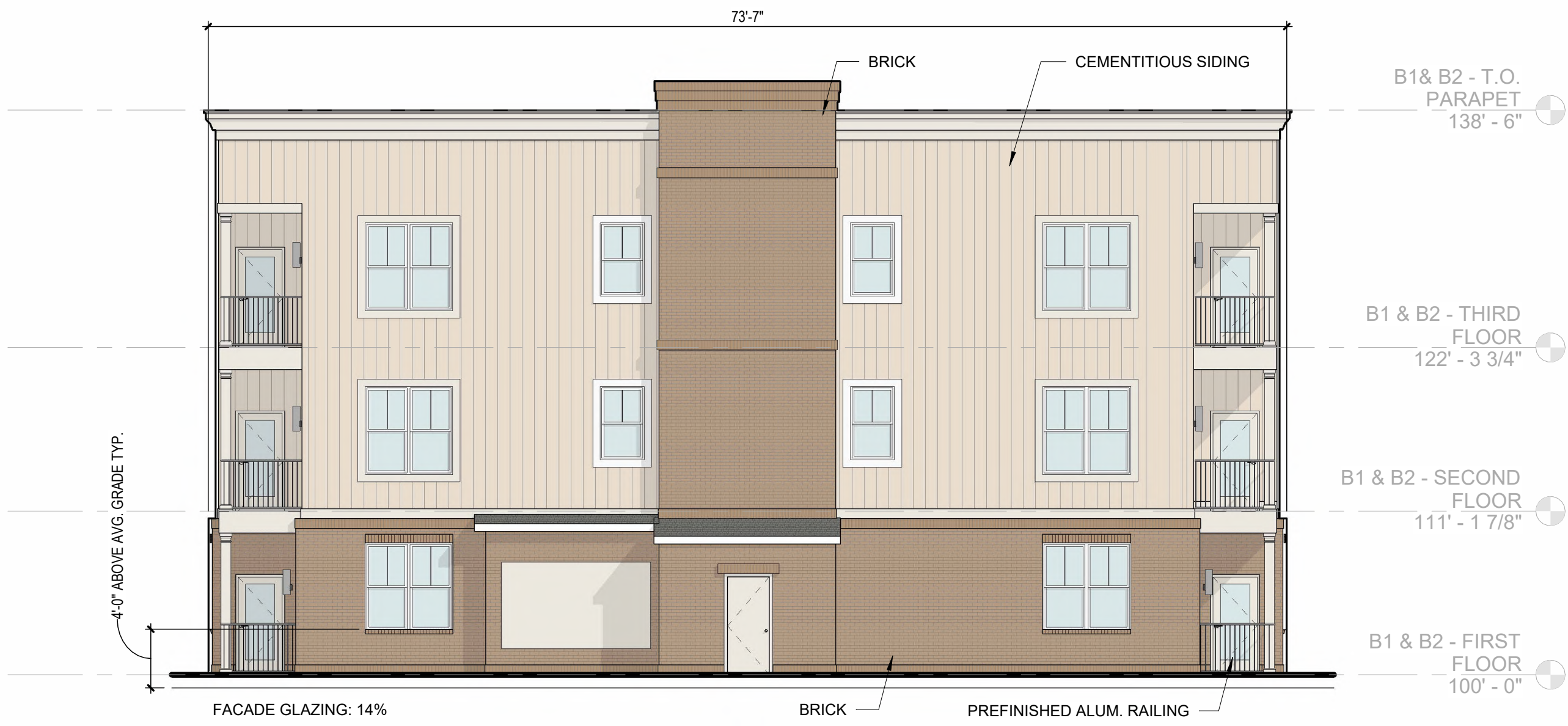
3 A201 1/8" = 1'-0" ELEVATION BUILDING 1&2 - (FACING BLDG 3)
