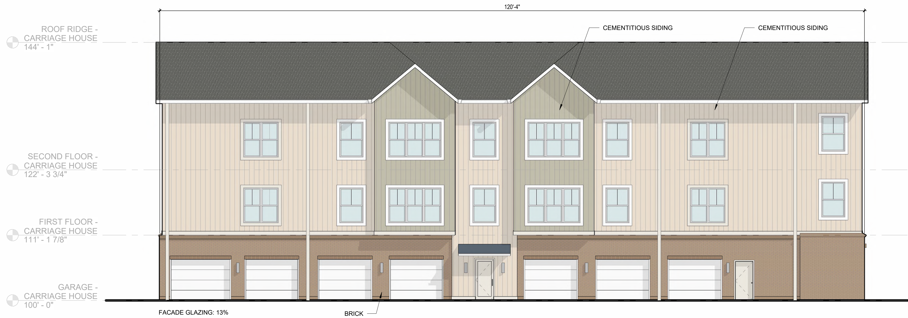
1 A205 1/8" = 1'-0" ELEVATION CARRIAGE HOUSE - (FACING PARKING LOT)
