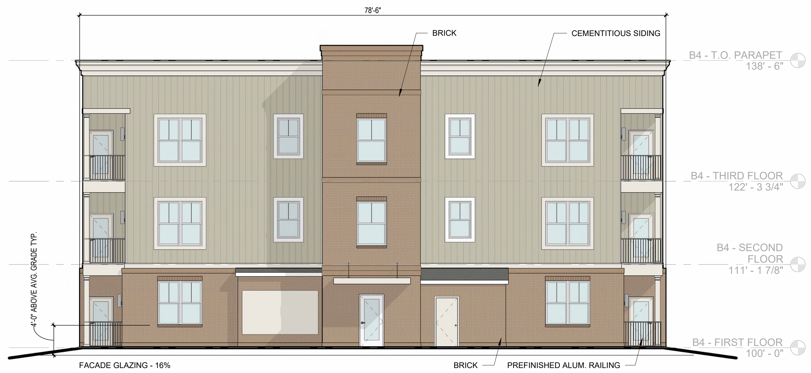
2 A203 1/8" = 1'-0" ELEVATION BUILDING 3 - (FACING PARKING LOT)
