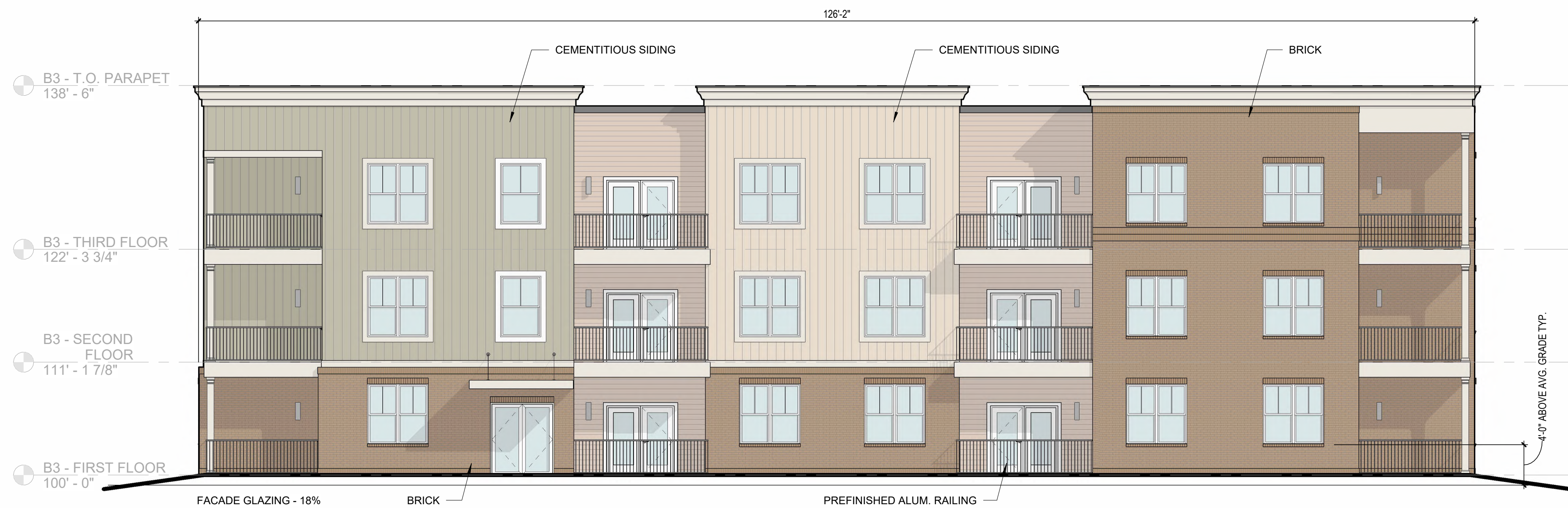
3 A203 1/8" = 1'-0" ELEVATION BUILDING 3 - (FACING BLDG 1&2)
