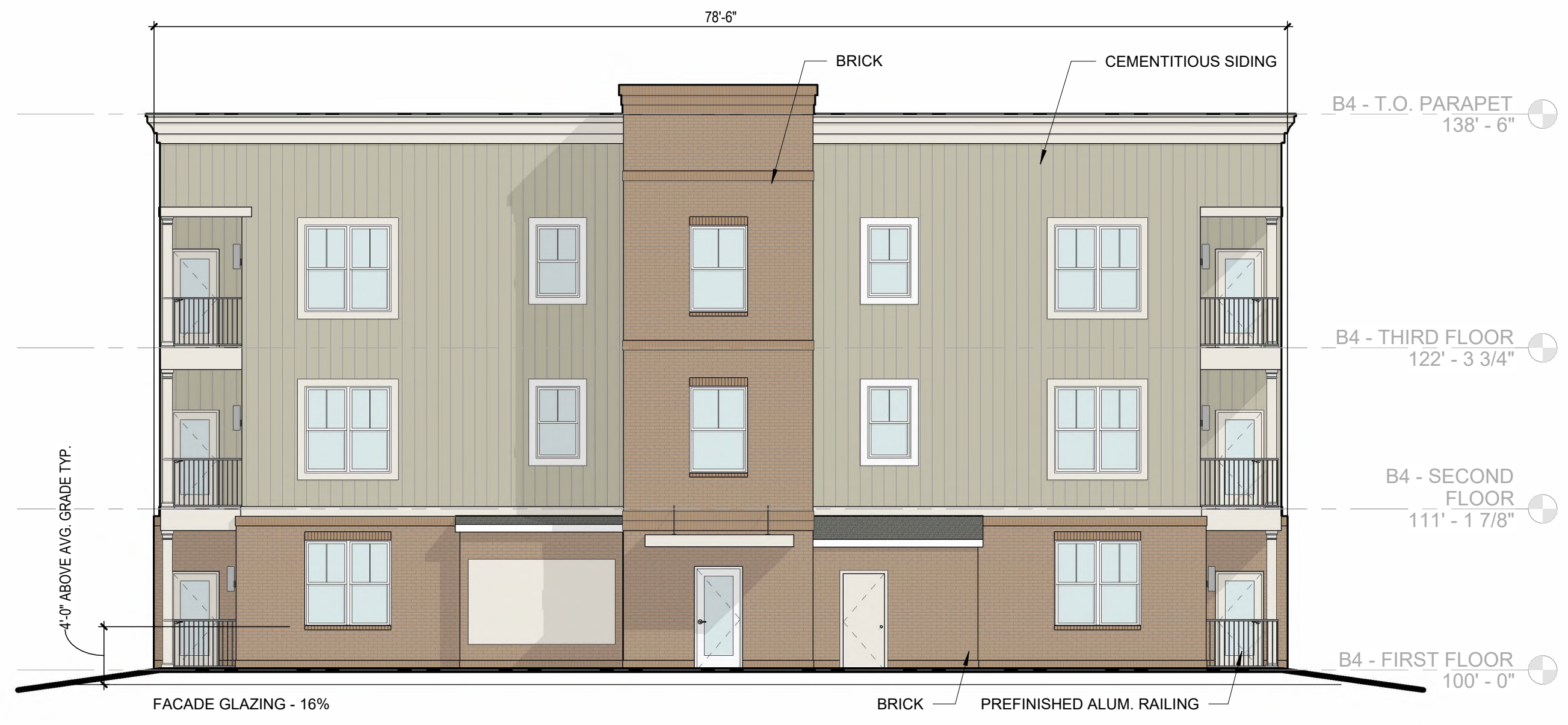
2 A203 1/8" = 1'-0" ELEVATION BUILDING 3 - (FACING PARKING LOT)
