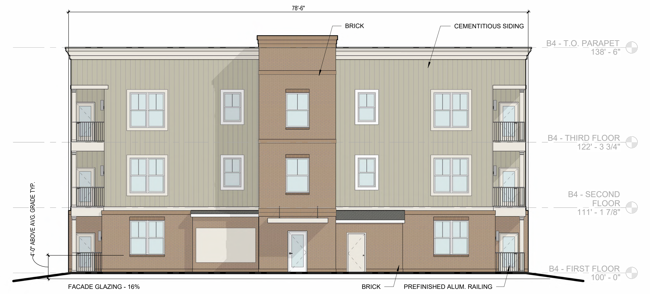
2 ELEVATION BUILDING 3 - (FACING PARKING LOT) A203 1/8" = 1'-0"
