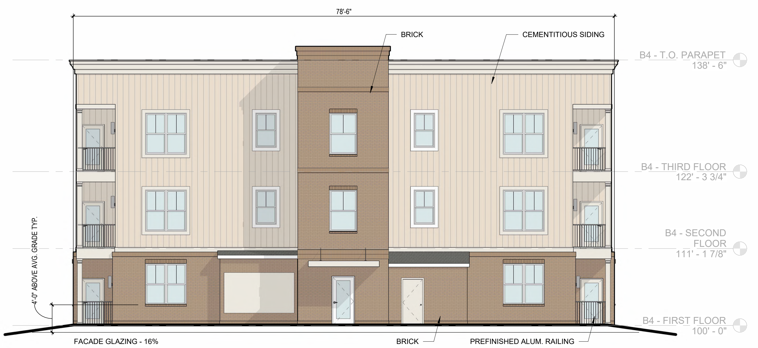
3 A204 1/8" = 1'-0" ELEVATION BUILDING 4 - (FACING BACK OF PROPERTY)
