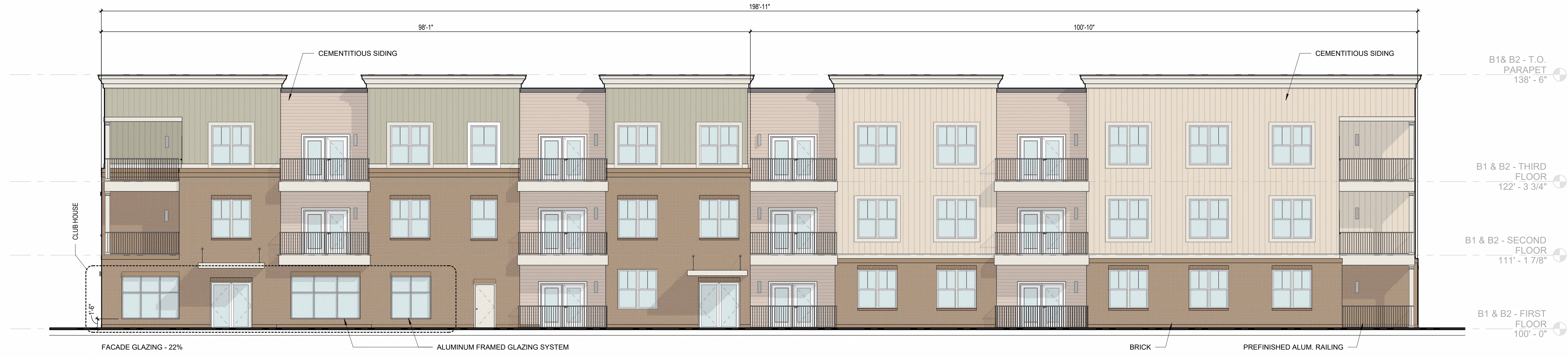
1 ELEVATION BUILDING 1&2 - (FACING RIVER RD.) A201 1/8" = 1'-0"
