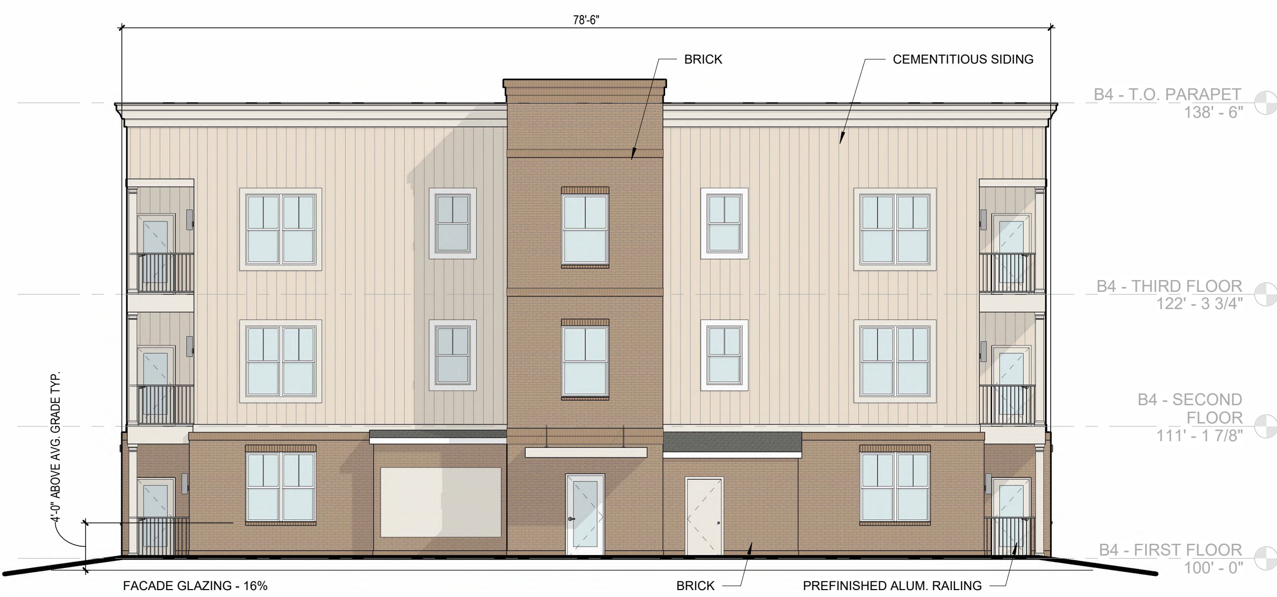
3 A204 1/8" = 1'-0" ELEVATION BUILDING 4 - (FACING BACK OF PROPERTY)
