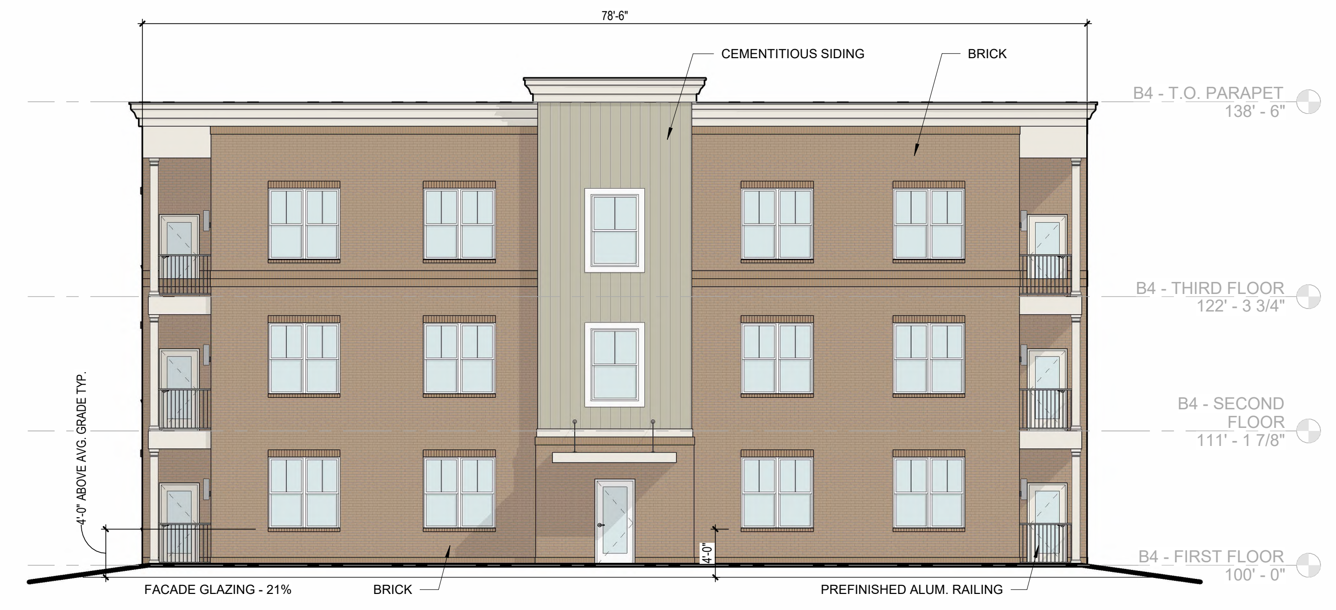
1 ELEVATION BUILDING 3 - (FACING RIVER RD.) A203 1/8" = 1'-0"
