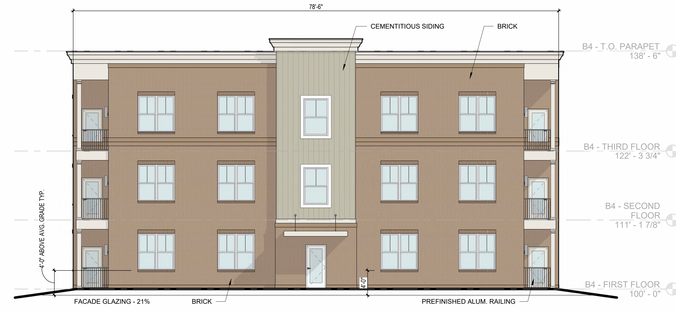
1 A203 ELEVATION BUILDING 3 - (FACING RIVER RD.) 1/8" = 1'-0"
