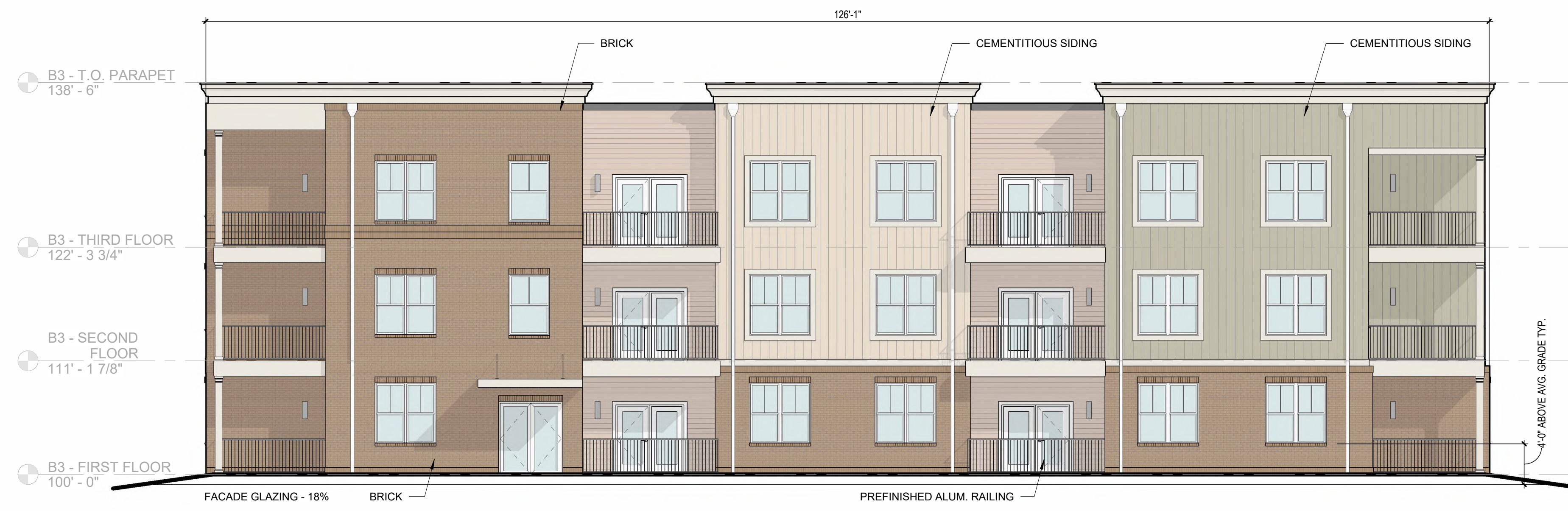
4 A203 ELEVATION BUILDING 3 - (FACING BACK OF PROPERTY) 1/8" = 1'-0"
