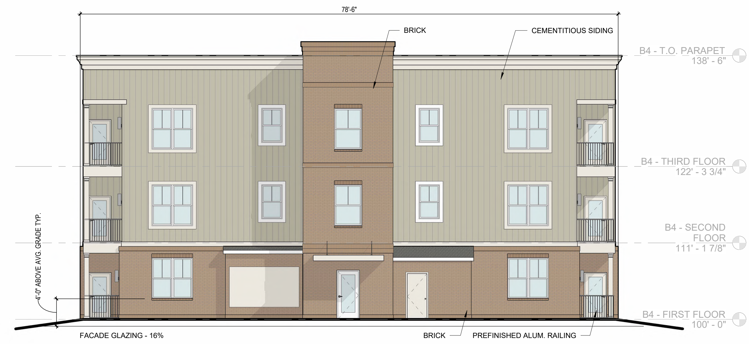
2 A203 ELEVATION BUILDING 3 - (FACING PARKING LOT) 1/8" = 1'-0"
