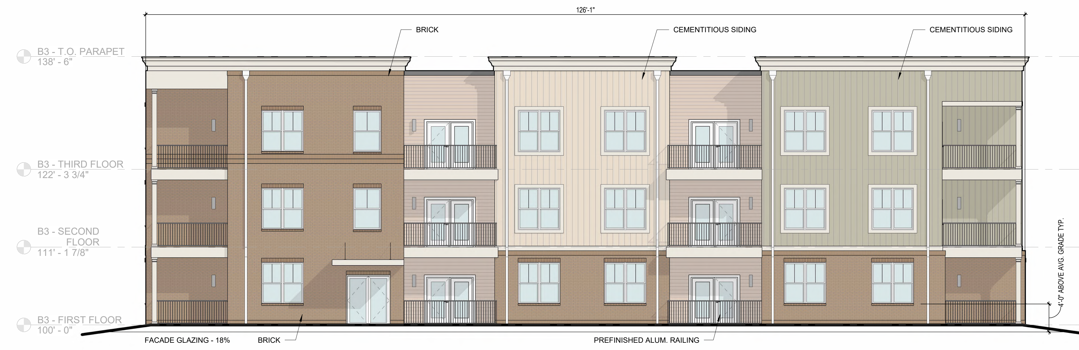
4 ELEVATION BUILDING 3 - (FACING BACK OF PROPERTY) A203 1/8" = 1'-0"
