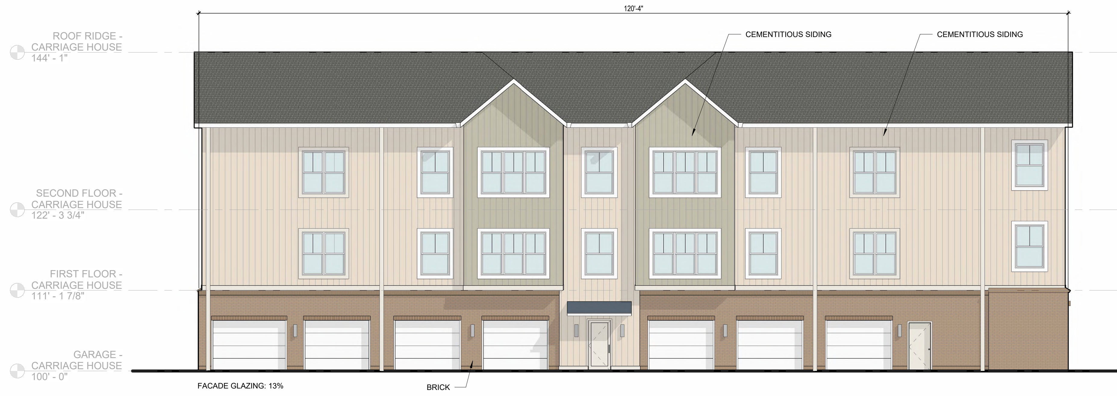
1 ELEVATION CARRIAGE HOUSE - (FACING PARKING LOT) A205 1/8" = 1'-0"
