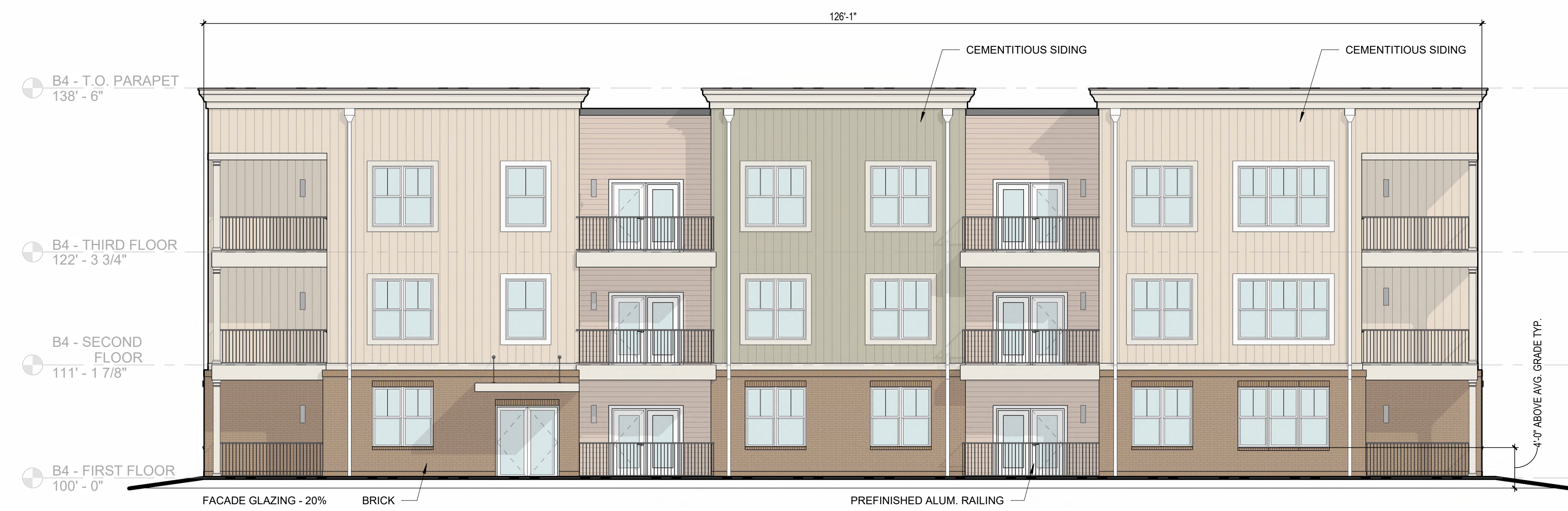
2 A204 1/8" = 1'-0" ELEVATION BUILDING 4 - (FACING WATER DETENTION AREA)
