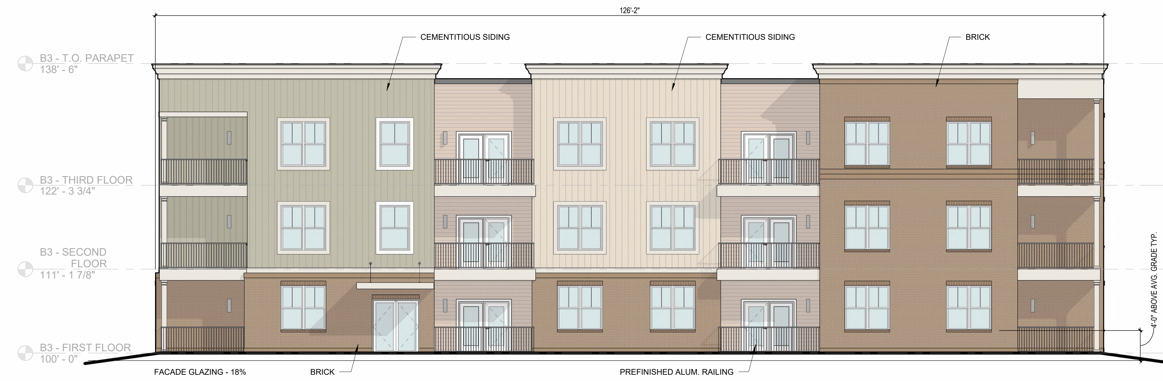
3 ELEVATION BUILDING 3 - (FACING BLDG 1&2) A203 1/8" = 1'-0"
