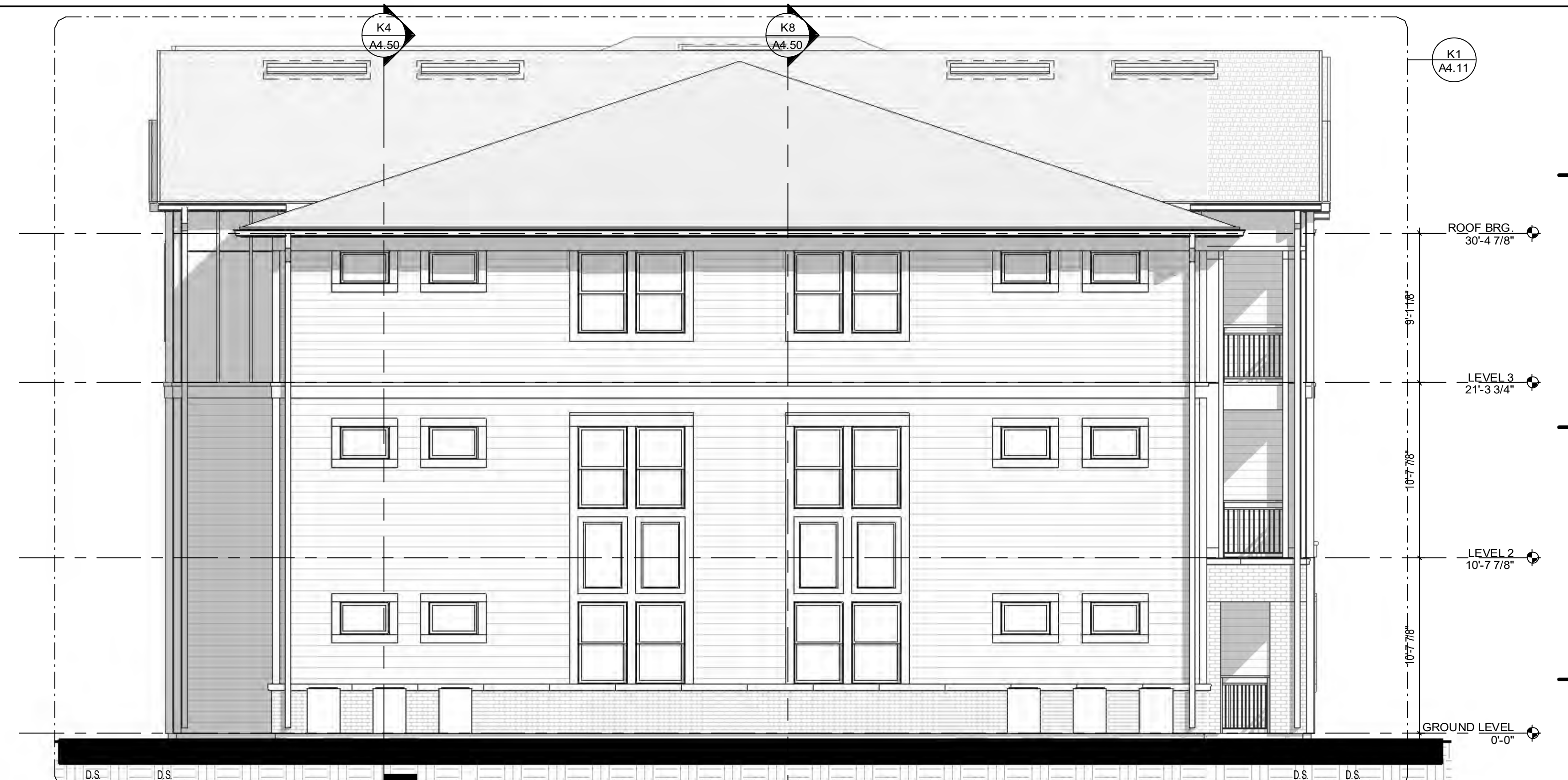
G7 BUILDING TYPE 1 - RIGHT SIDE ELEVATION 3/16" = 1'-0" E1/A2.01
