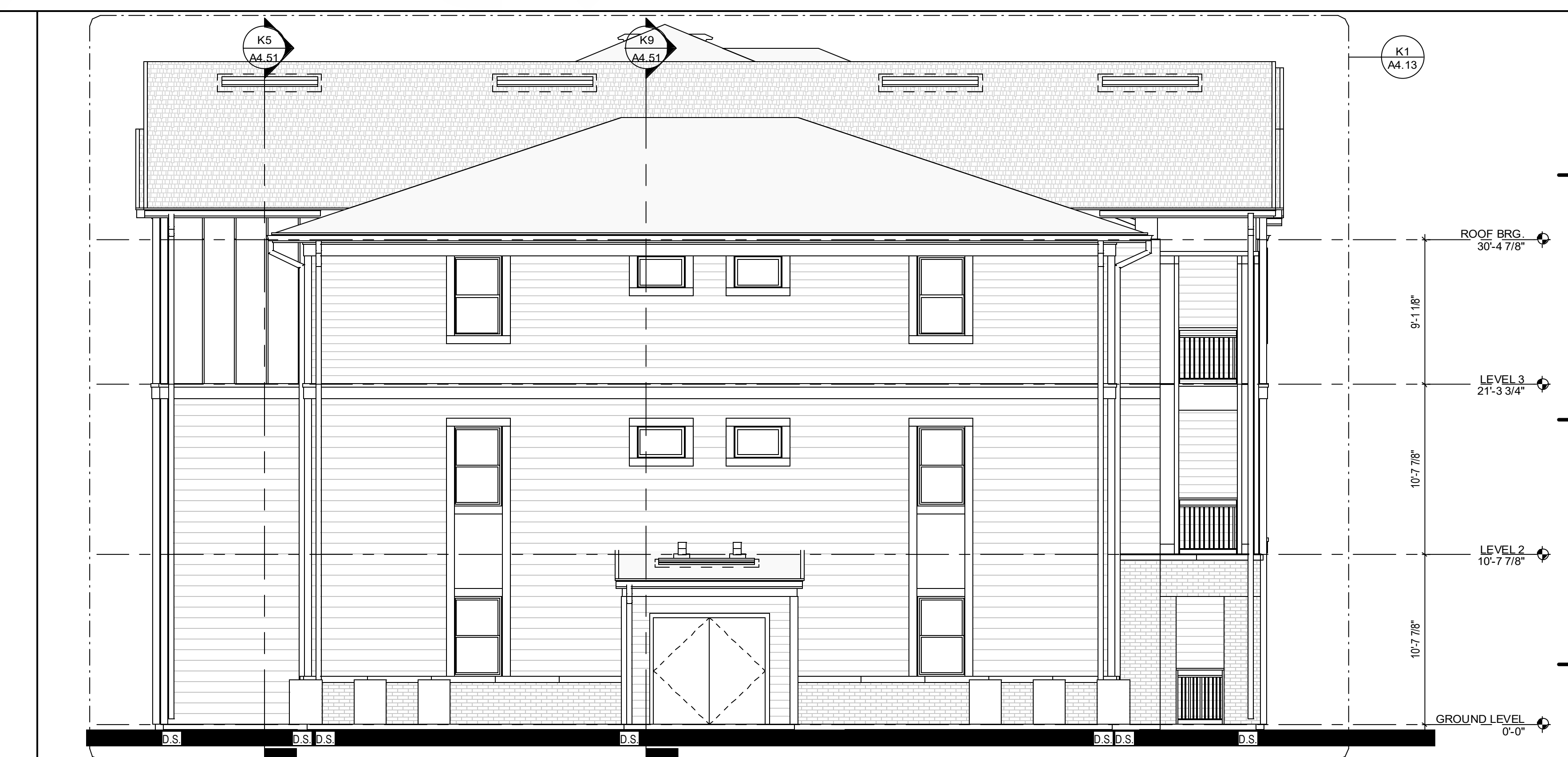
G7 BUILDING TYPE 2 - RIGHT SIDE ELEVATION 3/16" = 1'-0" E1/A2.03
