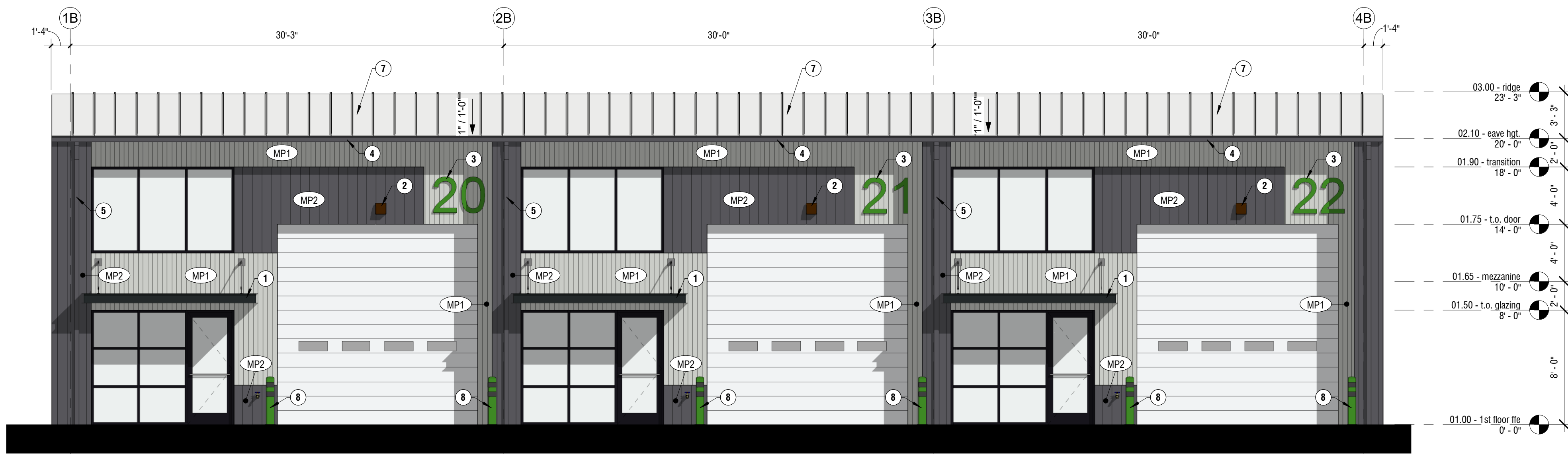
1 bldg type II - south elevation 3/16" = 1'-0"
