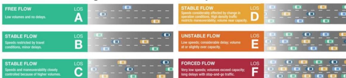
Figure 2: Illustration of Roadway Level of Service
